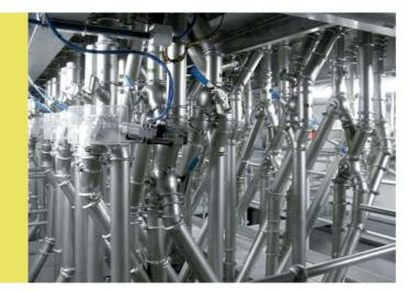
JACOB conveying pipe systems are used in a wide variety of industries for handling bulk materials or conveying products in downpipe systems.
